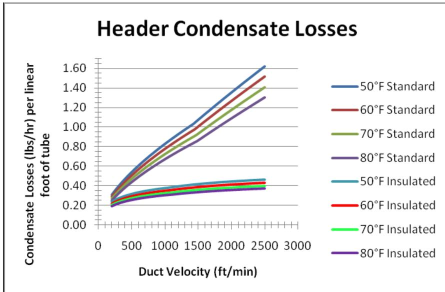
Figure 3: Condensate Losses per Linear Foot of Header
