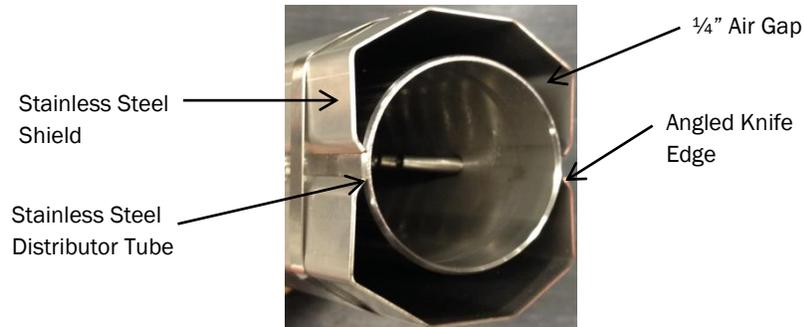
**Figure 1: Cross Section of Insulated Distributor Tube**
