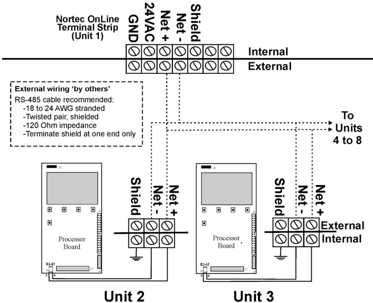
To network up to eight (8) units using a single Nortec OnLine module, the units must be connected in parallel (daisy-chained) to each other using the network link terminals supplied with Nortec OnLine equipped humidifiers.
